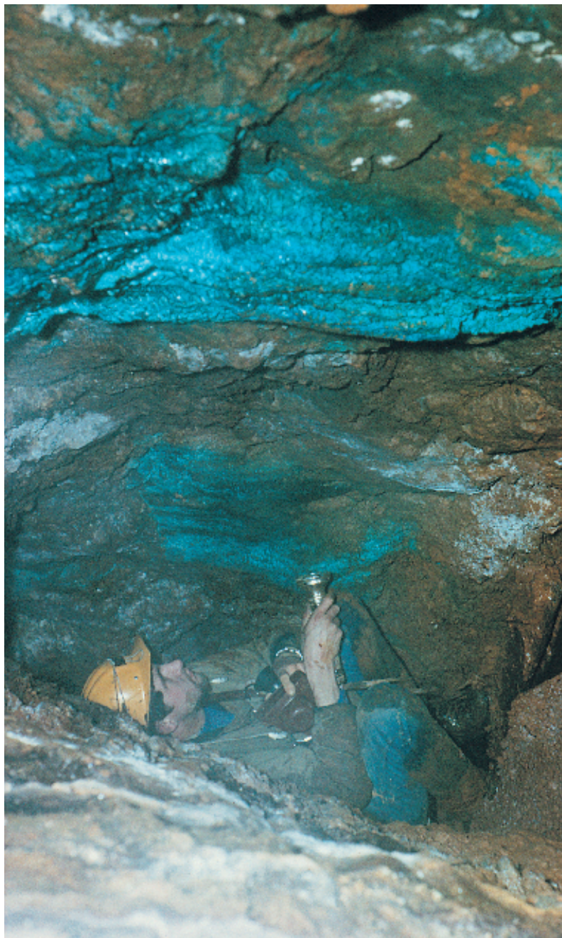
Plate 7. Secondary copper mineralization in a stope, Kenneggy Mine (part of Wheel Speed) [SW 565 285] (Photograph © A.J.J. Goode)
